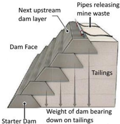
*“Upstream” tailings dam showing how the tailings form the foundation of the dam (acknowledgements to the journal “Science” 25 Dec 2020).*
